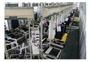
2 times leakage test of Titanium heat exchanger 3 times gas leakage test of the whole system
